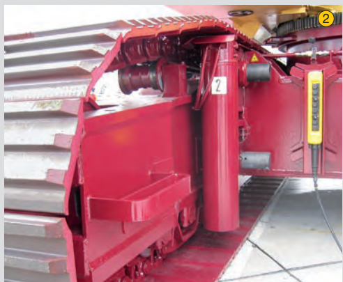
② Jack-up cylinders with retracted crawlers
