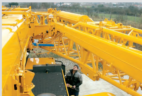
Hydraulic assistance for assembly of swing-away jib
